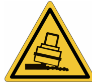
Risk of overturning during rolling
