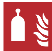
Remote release station
